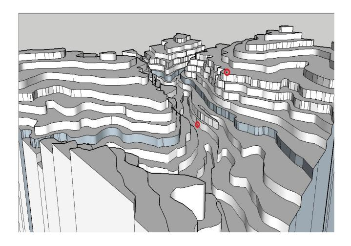
2. Topographic Model of Highway 14 and plateaus east of Cedar City, Utah. Upper red dot is surface location of a directional water well. Lower red dot is approximate point where directional well exits the subsurface.
