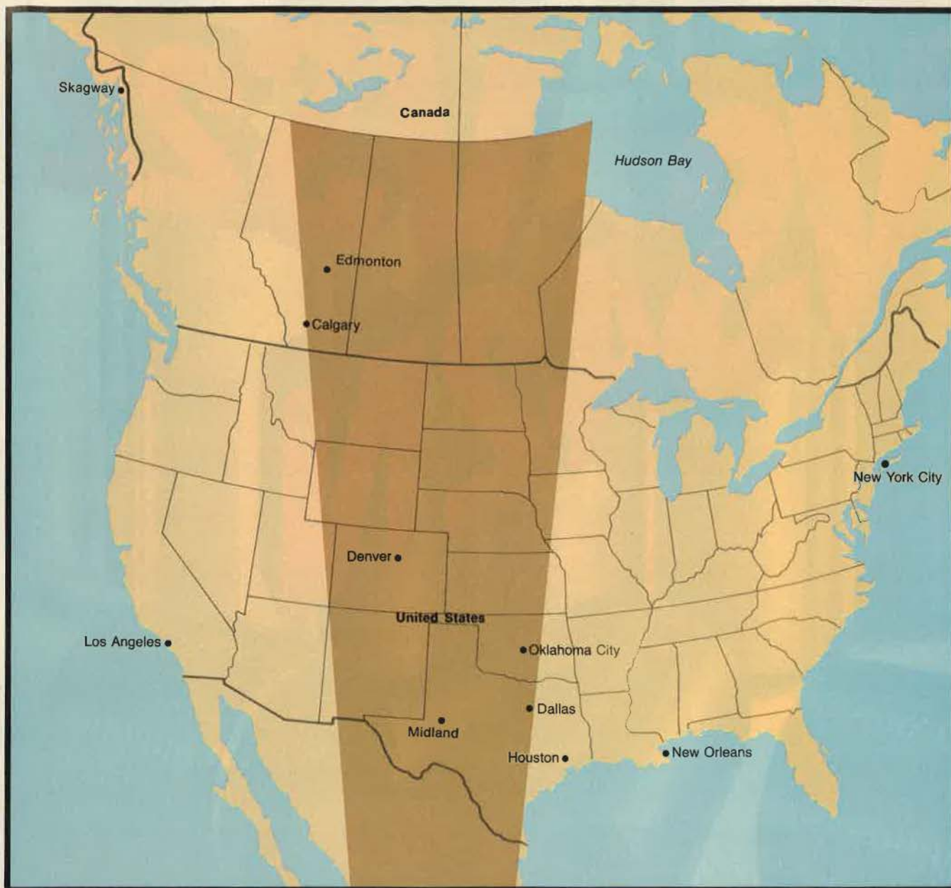
Fig. 8 —The ground communication coverage of the INMARSAT satellites. Note the large gap in coverage that excludes Oklahoma City, Denver and Calgary from receiving signals directly from INMARSAT. To transmit data to the areas within the gap, information must be re-sent through another satellite. This is just one of the problems that have kept satellite data transmission out of the oil patch.
