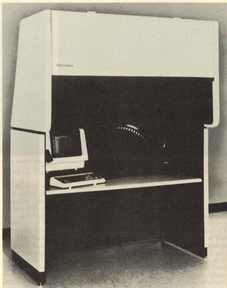
Fig. 10—The Genisco SpaceGraph vibrating mirror 3D display device. A 40-cm vibrating mirror is partially shown at the center of the display. A high-resolution CRT is housed within the overhead casing.
