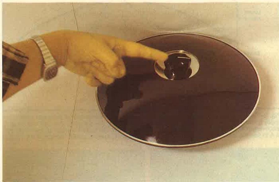
Fig. 1 —In this simple 3D imaging device, called the Mirage, two parabolic mirrors face each other and are separated by the distance of their common focal lengths. Note that the hole being pointed to acts as a mirrored surface, and that even the imaged object, the knob also pointed to, is actually resting in the bottom of Mirage although it appears to be reflected on the mirror. (See Fig. 2).
