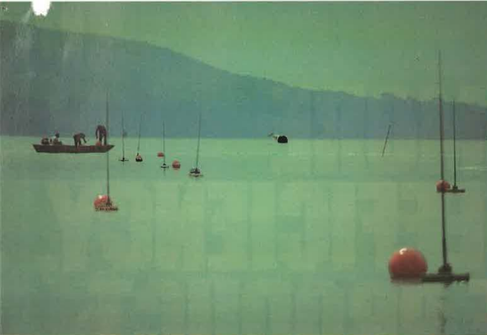
Fig. 3 —A TELSEIS radio system at work in the field. Each channel utilized (up to a maximum of 66 channels) has a separate radio frequency. It can be operated from land or in shallow to deep water zones without equipment change.
