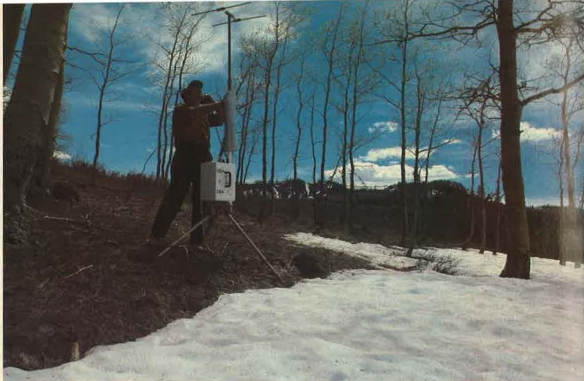
Fig. 1—Observer talking to the recording truck from an OPSEIS Remote Telemetry Unit. These units are essentially four-channel, portable, digitizing boxes designed to relay seismic data without the use of wires.
