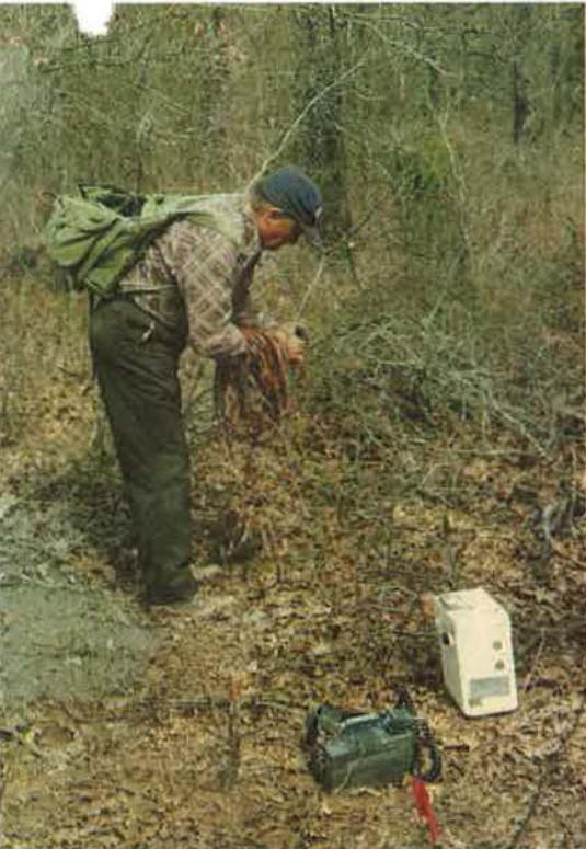
Fig. 2 —An SGR cassette cartridge system being placed in the field. A single channel is recorded on the tape for every shot or vibrator point. Data from the individual tapes are dumped onto a larger system at day's end.
