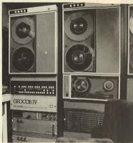
Advanced computer hardware allows the GEOCOR IV to demultiplex, correlate and composite results for display on the system plotter during parameter testing for immediate, on-site evaluation, and during data acquisition for "real-time" monitoring of data quality.
