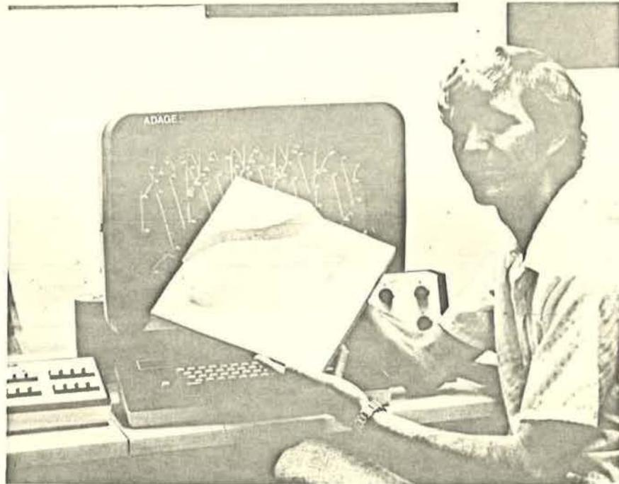
Figure 1. Physical Model SALGLF and line drawing display terminal with raster segment generator.
