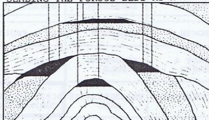
RENEWED UPLIFT DEFORMS BEDS ABOVE THE UNCONFORMITY CREATING ADDITIONAL RESERVOIRS
