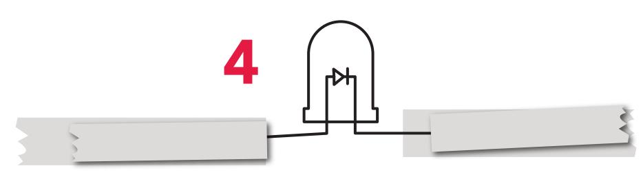
Now cover the ends of the leads with little pieces of copper tape. Press the tape down very well.
