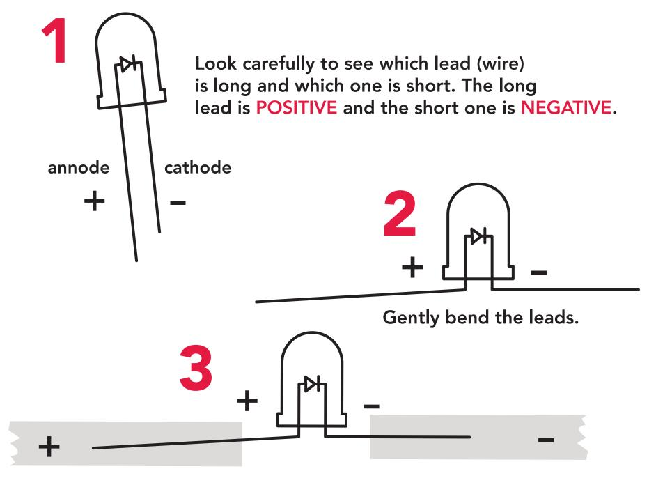
Place the LED onto the copper tape. Be sure to match positive with positive and negative with negative.
