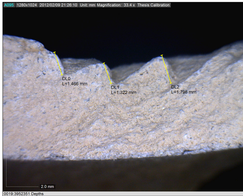
Figure 41. Micrographs of sherd 0019-395-2351 taken using a Dino-Lite Pro AM413T at 33.4x magnification: a) measurement of indent angles in degrees; and b) measurement of indent depths in millimeters.
