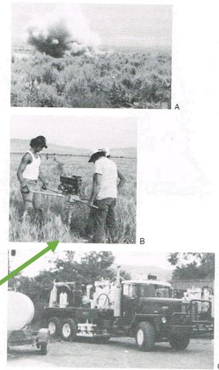
Figure 1-5. Typical land crew operations in southwestern Utah. (A) Surface shooting using ten 5-lb sacks of explosives on a primachord string. The environmental damage is temporary, but overgrazing, like overgrazing, can cause long-term problems. (B) Shallow hole shooting of, say, 10 lbs of dynamite per shotpoint is better in agricultural areas. (C) The most common land seismic source is Vibroseis.™ Normally, four of these trucks vibrate in synchronization.
