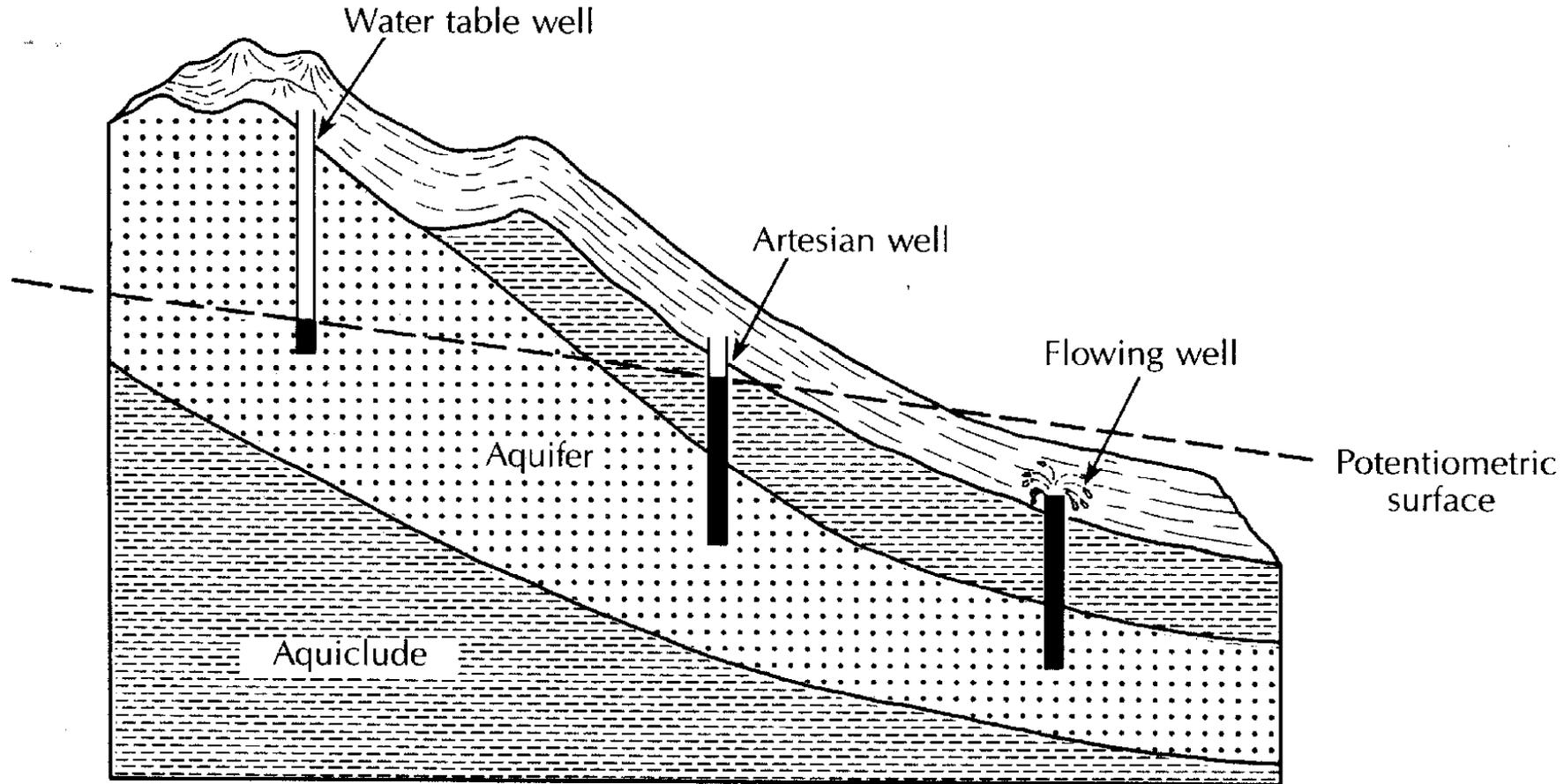
**FIGURE 4.21** Artesian and flowing well in confined aquifer.
