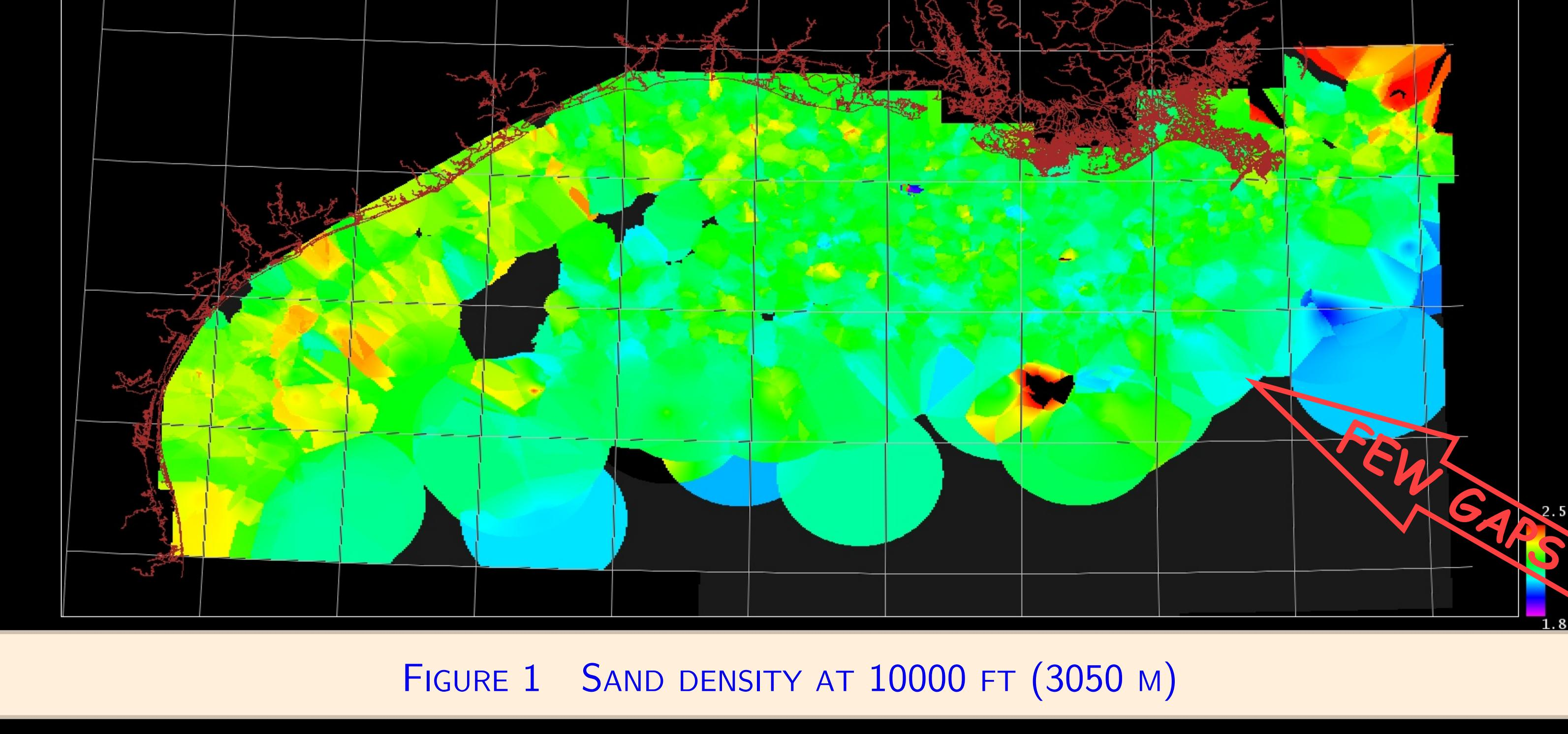
FIGURE 1 SAND DENSITY AT 10000 FT (3050 M)
