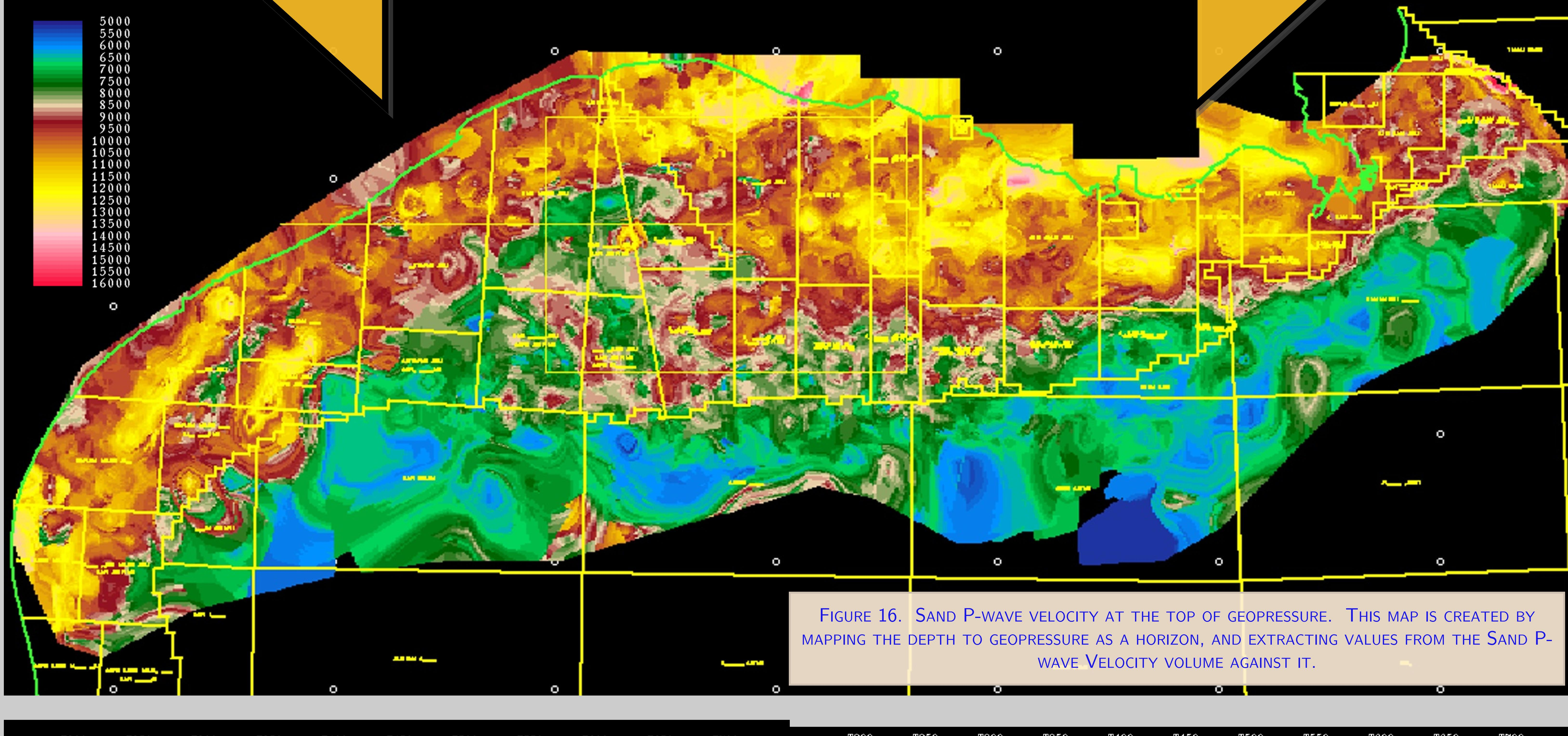
FIGURE 16. SAND P-WAVE VELOCITY AT THE TOP OF GEOPRESSURE. THIS MAP IS CREATED BY MAPPING THE DEPTH TO GEOPRESSURE AS A HORIZON, AND EXTRACTING VALUES FROM THE SAND P-WAVE VELOCITY VOLUME AGAINST IT.
