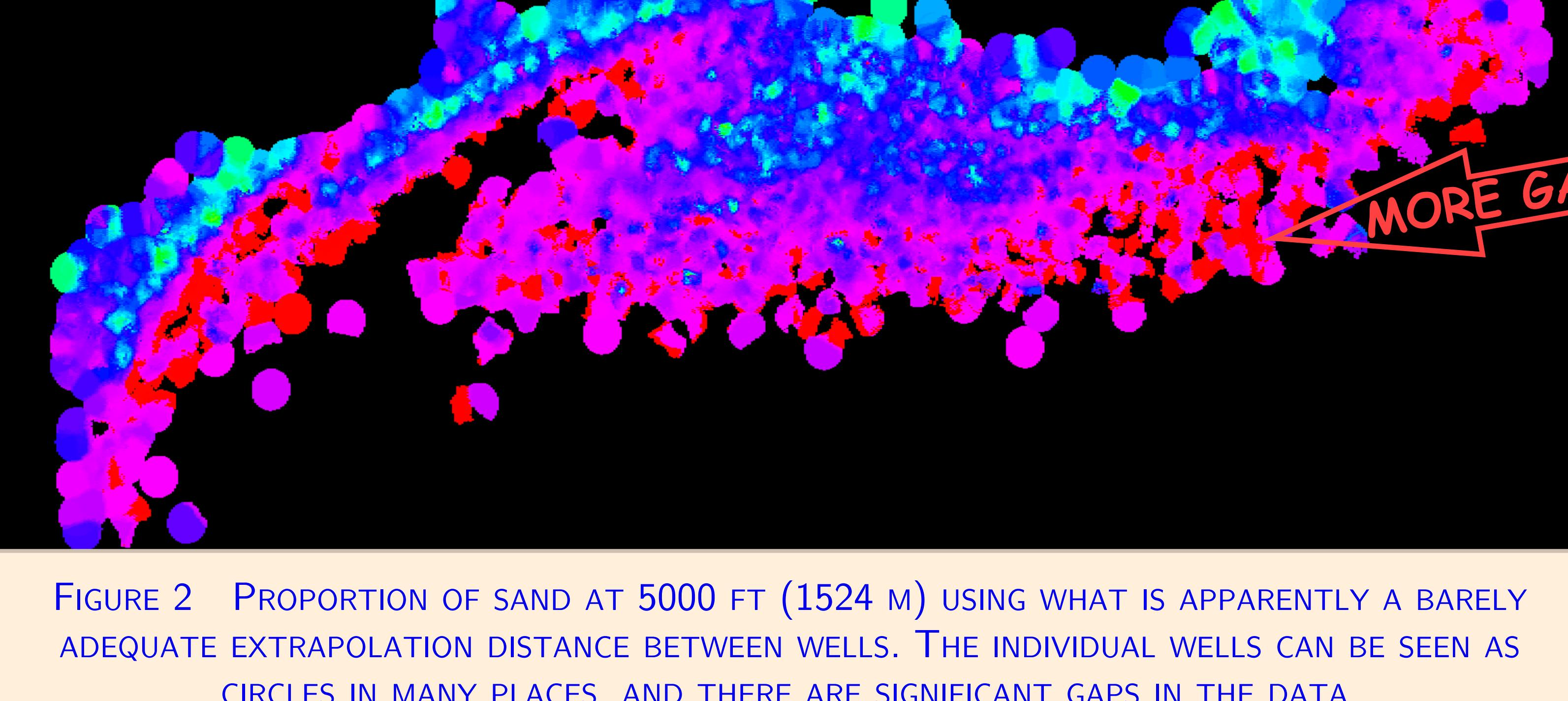
FIGURE 2 PROPORTION OF SAND AT 5000 FT (1524 M) USING WHAT IS APPARENTLY A BARELY ADEQUATE EXTRAPOLATION DISTANCE BETWEEN WELLS. THE INDIVIDUAL WELLS CAN BE SEEN AS CIRCLES IN MANY PLACES, AND THERE ARE SIGNIFICANT GAPS IN THE DATA.
