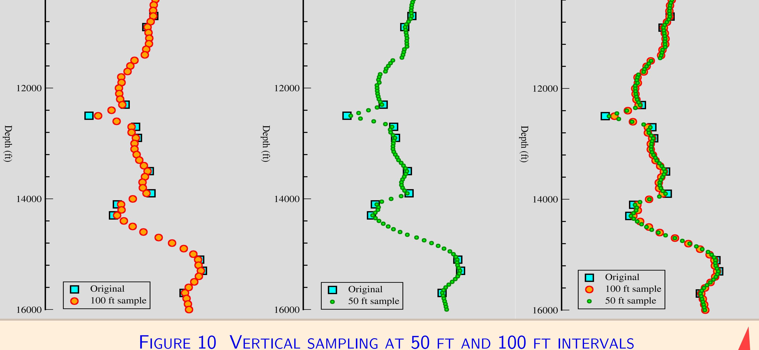
FIGURE 10 VERTICAL SAMPLING AT 50 FT AND 100 FT INTERVALS
