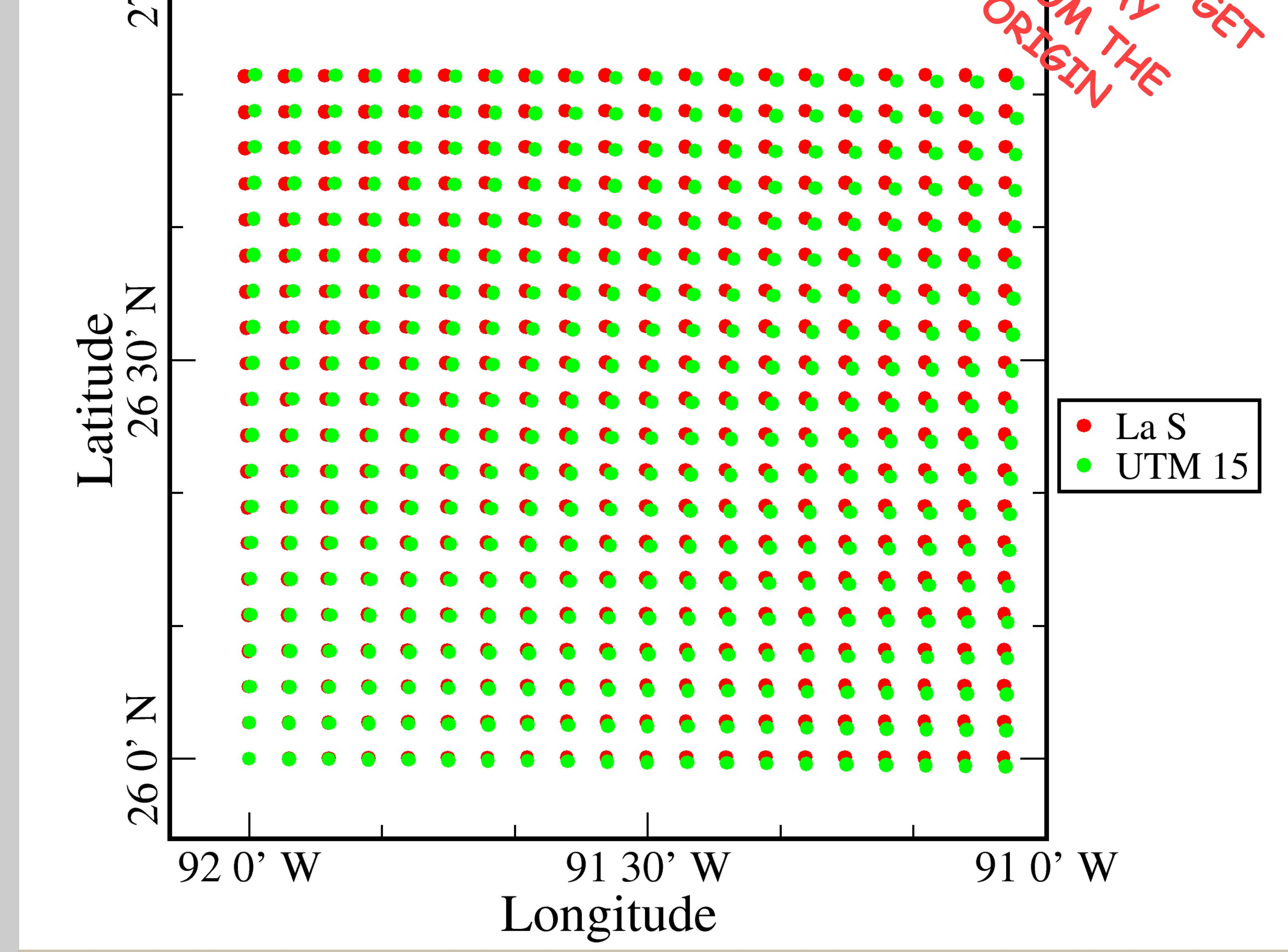
FIGURE 4 BIN CENTERS COMPUTED ON TWO DIFFERENT PROJECTIONS: LOUISIANA SOUTH STATE PLANE, AND UNIVERSAL TRANSVERSE MERCATOR ZONE 15
