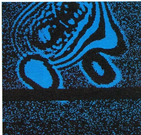
Figure 4-8. Interactive 3D interpretation techniques are becoming much more common. Here two horizontal sections across the SALGLF model are shown (A and B). There is no data in the black strip because of a data collection error.
