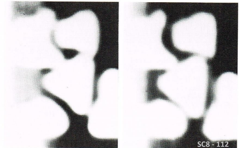
Figure 8-7. A stereoscopic projection of a volume of Hilbert Transformed 3D migrated data from the physical model in Figure 8-5. Note the focusing effect of migration compared to Figure 8-6. 24
