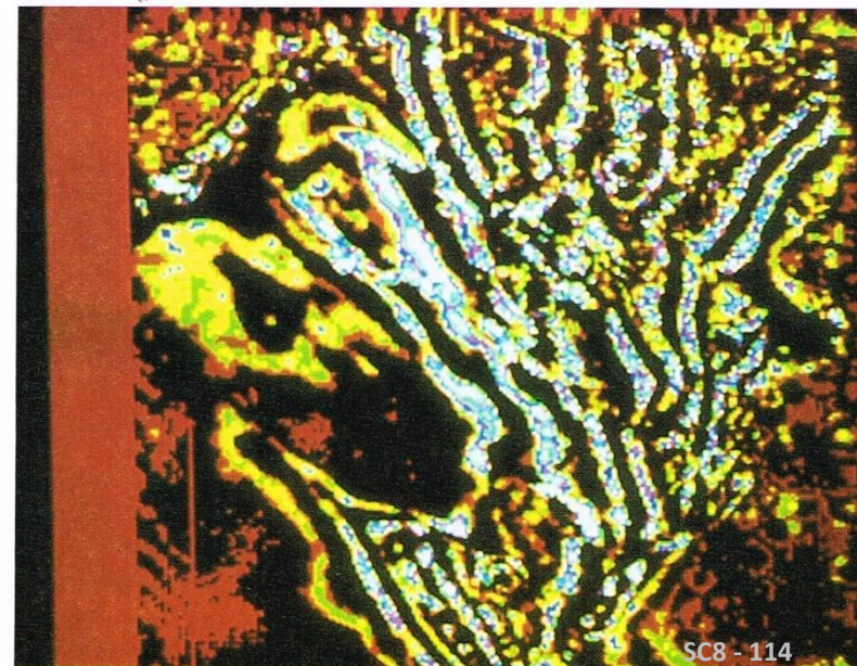
Figure 6-13H. A time-slice section from the same SALNOR 3D survey at time 1.22 seconds. At this depth the section cuts through the two dipping, producing Brent and Statfjord sandstones. The fault cuts are easily identified, especially when a sequence of time-slices are animated like a movie.
