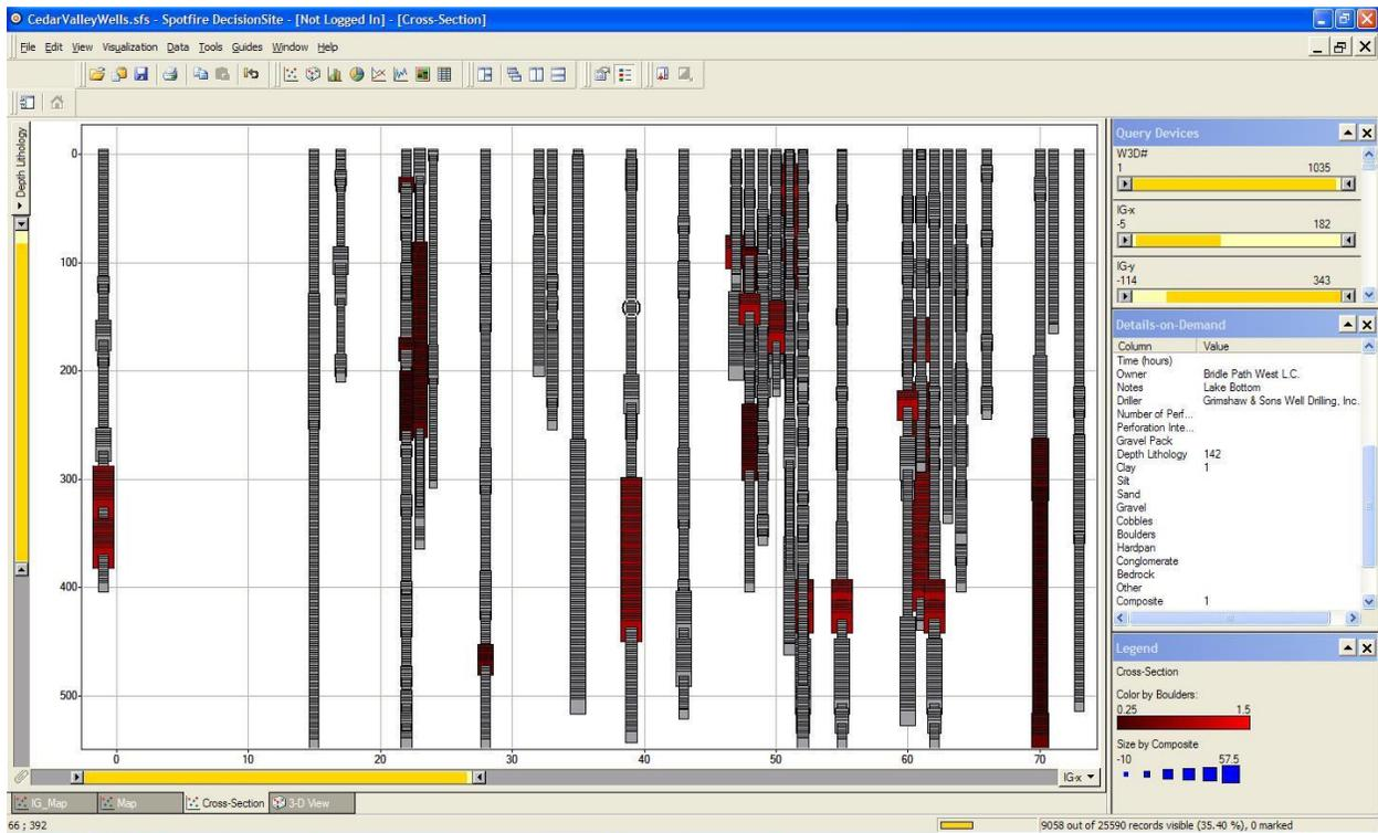
Figure 9. Boulders on the west end of the West-to-East cross-section through the Cedar Valley Aquifer.
