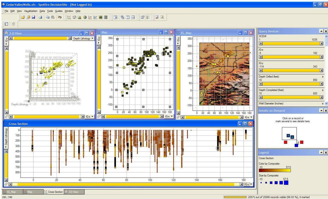
Figure 3. West-to-East cross-section showing wells in the Cedar Valley Aquifer.
