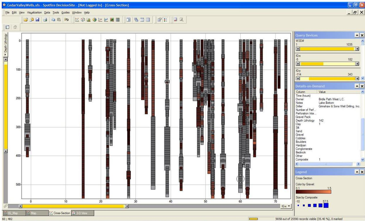
Figure 7. Gravel on the west end of the West-to-East cross-section through the Cedar Valley Aquifer.
