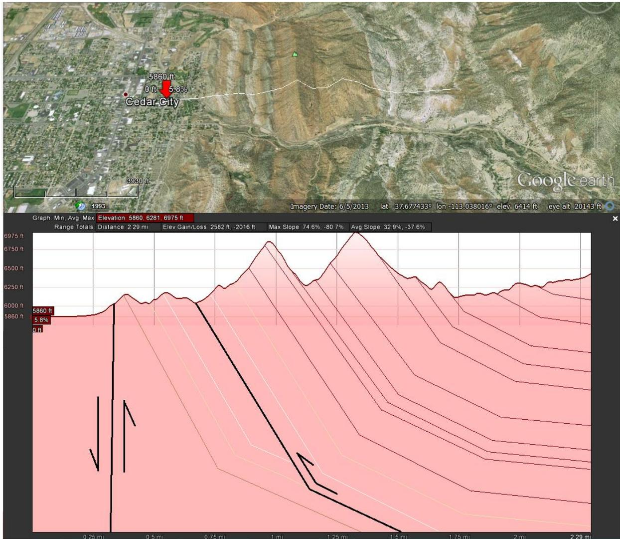
Figure 21. Thrust structure underneath the Red Hills.
