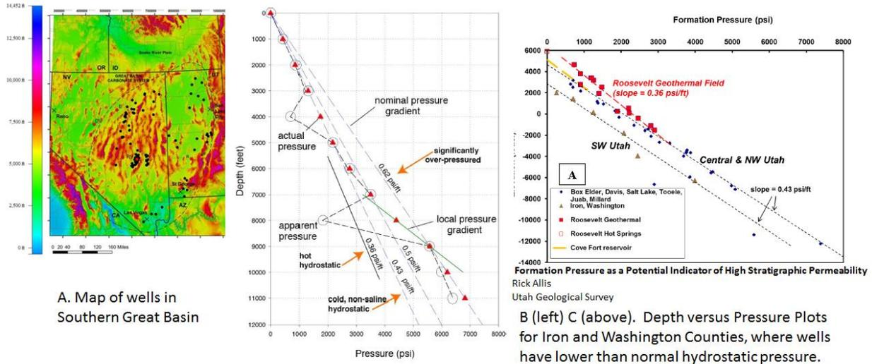
Figure 13. A. Map of wells showing hydrostatic pressure in the Southern Great Basin. B. Plot of normal pressure gradient as water builds up in the subsurface, and the actual pressure gradient for wells in the southern part of the Great Basin. C. Pressure gradients for geothermal wells and water wells in Washington and Iron Counties, Utah.
