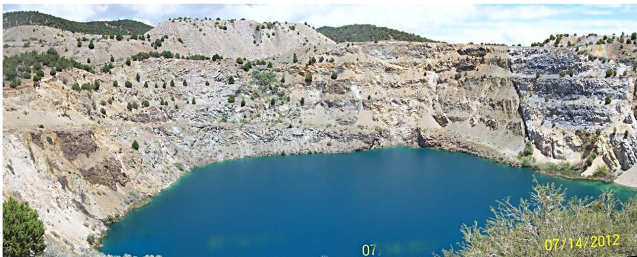
Figure 17. Shows the extent of water coming out of the fractured quartz monzonite at Blowout Pit at Iron Mountain.
