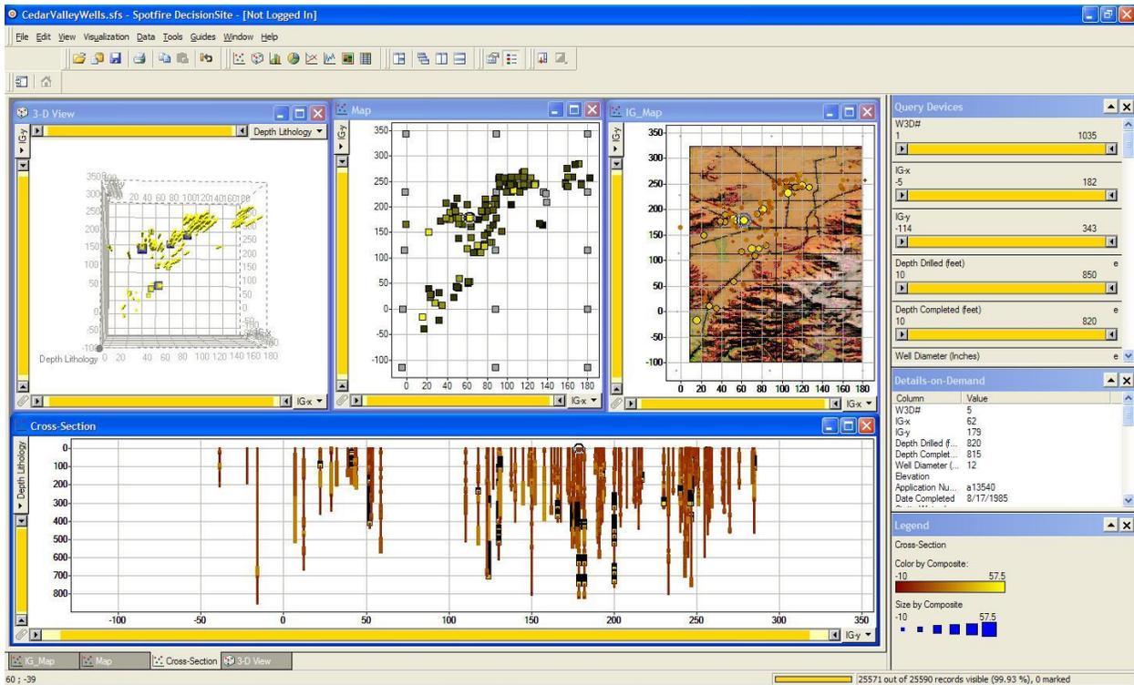
Figure 2. North-to-South cross-section showing wells in the Cedar Valley Aquifer.
