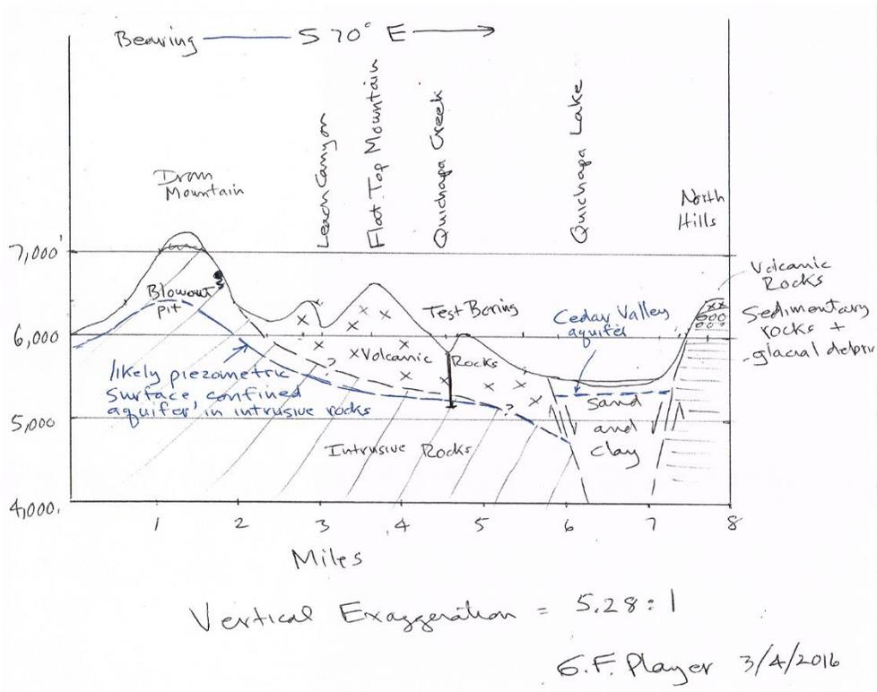
Figure 19. Cross-Section from Blowout Pit to North Hills on the other side of the Cedar Valley Aquifer.
