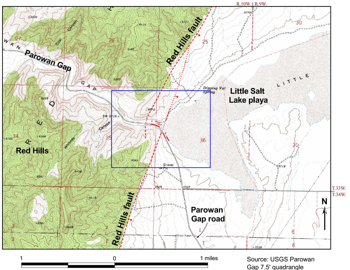
Figure 2. Western Parowan Valley, along the western margin of the Little Salt Lake playa. Solid red lines represent ground cracks. Red dashed and dotted lines indicate inferred location of the Red Hills normal fault; ball and bar on downthrown side (modified from Maldonado and Williams, 1993). Blue box indicates extent of figure 3.
